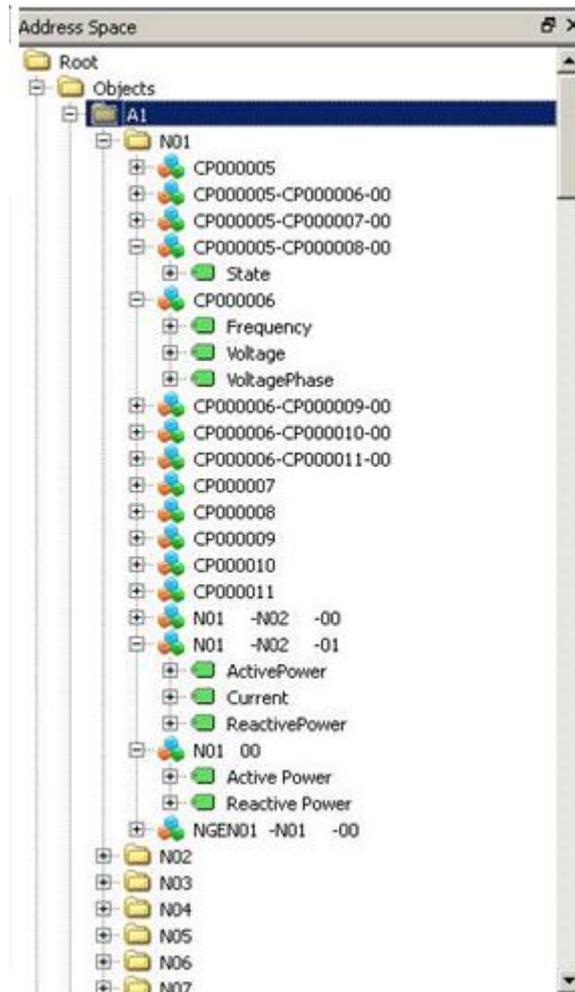
Figure 5-3: Observables access through a standard OPC UA client browser
